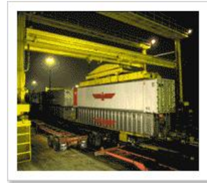
Containers being loaded onto stackcars.
